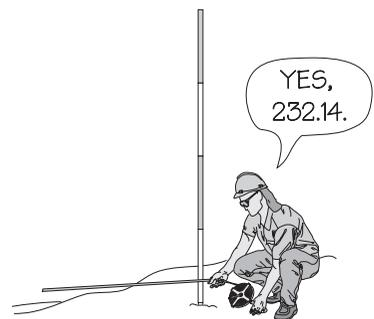
**Step 15** The distance measured is the total of the number of chain lengths measured plus the reading the head chain made at the last measurement.
