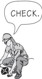
**Step 7** Rechecks alignment and makes sure ZERO was being held on the point.
